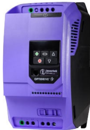
7.5HP VFD for 60GPM Pump Indoor
